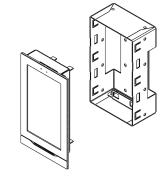
First, the mounting box must be attached to a suitable place on the wall. The long side of the mounting box should be placed at a right angle to the ground.
