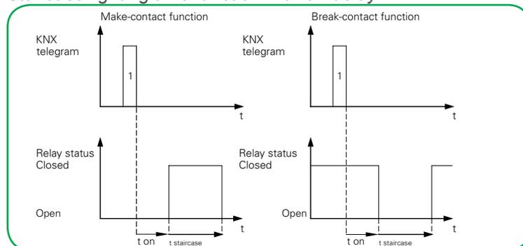
The result of combining a staircase lighting time function with an off-delay depends on how you have defined the staircase lighting time function:
